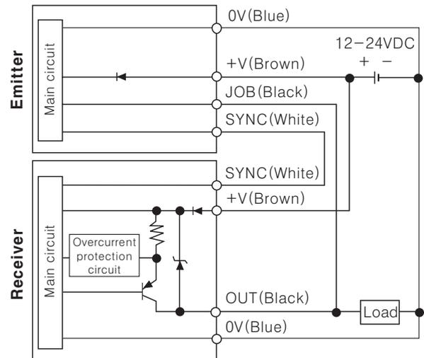
※If the receiver OUT(Black) line and the emitter JOB(Black) line are not connected each other, the JOB indicator of the emitter is not operated and maintain the light status.
